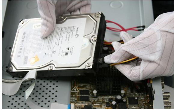
Figure 1.8 Connect the power cable
