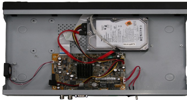
Figure 1.9 Place the HDD on the bottom
